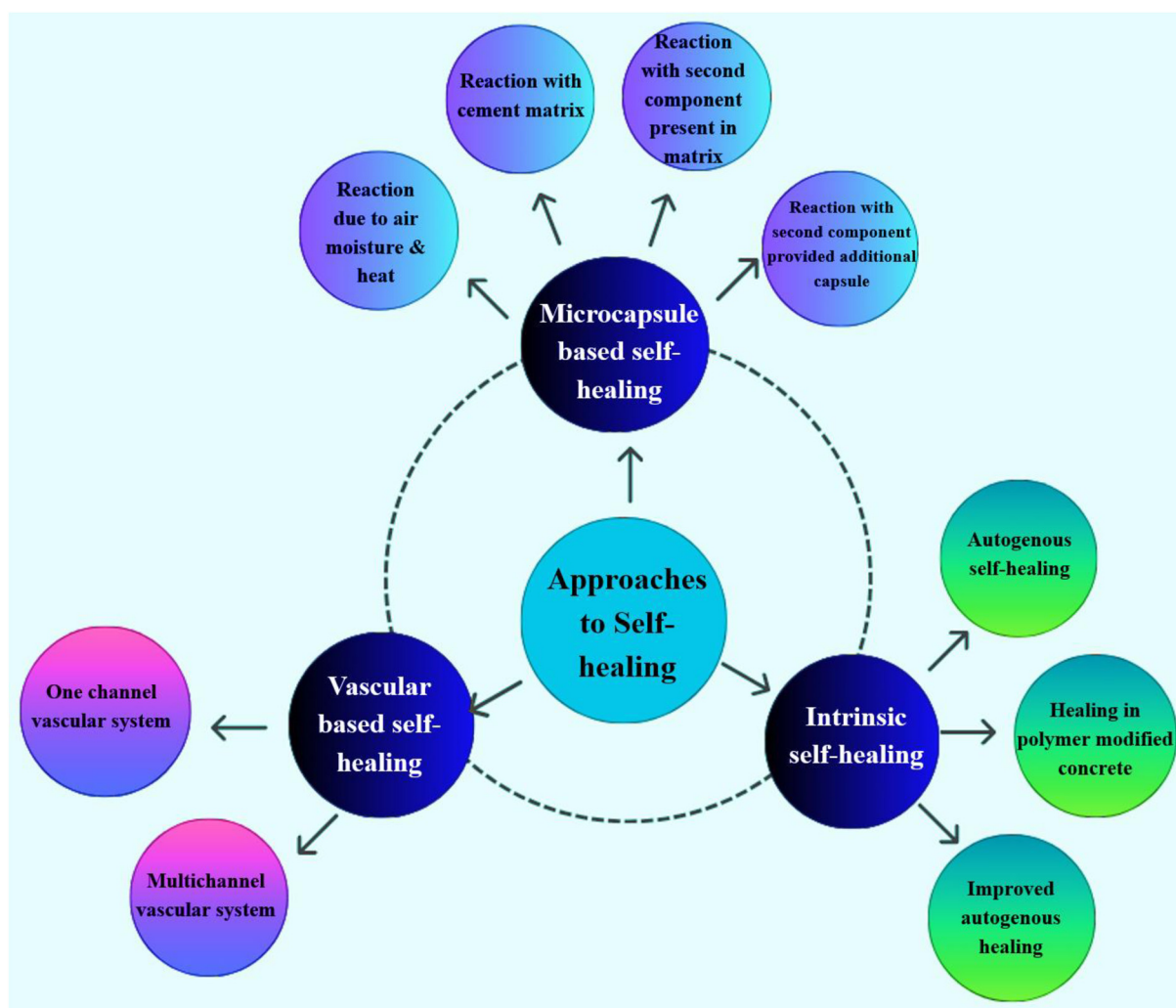
Fig. 3 Types of self-healing strategies in concrete materials.
