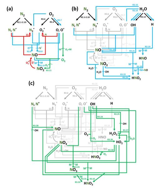
Fig. 2 Reaction diagrams of the  $N_2$  oxidation processes in (a)  $N_2$ :  $O_2$  (air), (b)  $N_2 + H_2O$  and  $N_2 + O_2$  (air)  $+ H_2O$  feedstocks, where (c) highlights the chemistry in the plasma/liquid interface. Black, blue, red, and green arrows indicate electron impact reactions, forward reactions, reverse reactions at high temperature, and reactions pronounced at low temperature, respectively.
