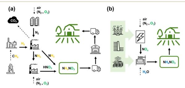
Fig. 1 Schematic representation of the fertilizer production and delivery chain for HB-based (a) and plasma-based (b) NH<sub>4</sub>NO<sub>3</sub>. The plasmabased route used as an example here involves electrocatalytic reduction as one step to directly obtain an aqueous solution of NH<sub>4</sub>NO<sub>5</sub>.
