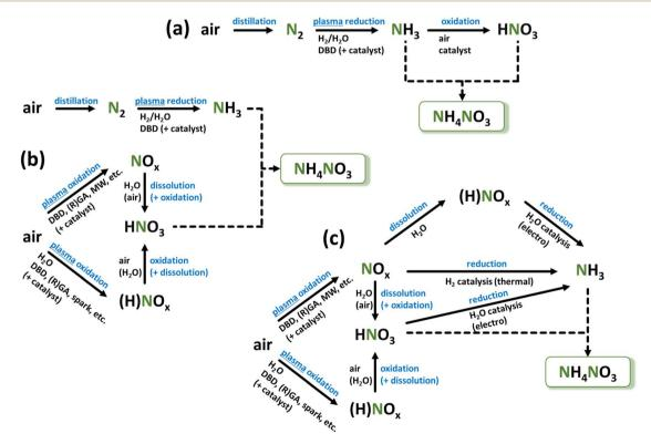
Fig. 5 Pathways of  $NH_4NO_3$  production via plasma-based NF: (a) plasma production of  $NH_3$  coupled with its subsequent (partial) oxidation to  $HNO_3$ ; (b) plasma production of  $(H)NO_x$  coupled with plasma-based production of  $NH_3$ ; (c) plasma production of  $(H)NO_x$  coupled with its subsequent (partial) reduction to  $NH_3$ .
