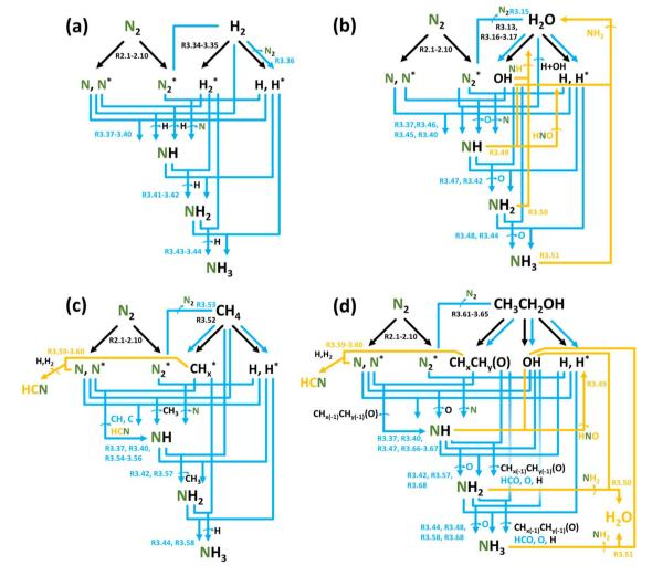
Fig. 3 Reaction diagrams of the  $N_2$  reduction processes in (a)  $N_2$ :  $H_2$ , (b)  $N_2 + H_2O$ , (c)  $N_2 + CH_4$ , (d) and  $N_2 + EtOH$  feedstocks. Black, blue, and yellow arrows indicate electron impact reactions, forward reactions, and reverse reactions, respectively
