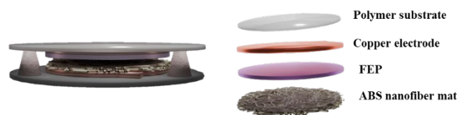
Figure 2. Schematic representation of ABS-based TENG
