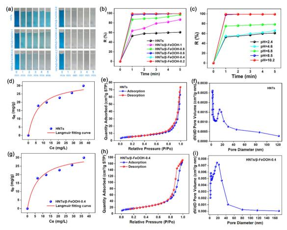
Fig. 4 (a) Photographs of the adsorption effect of powder HNTs/ $\beta$ -FeOOH-x on MB solution (20 mg L<sup>-1</sup>) within 5 min. (b) Removal rate of MB by HNTs/β-FeOOH-x. (c) Removal rate of MB by HNTs/β-FeOOH-0.4 from solutions (20 mg L<sup>-1</sup>) at different pH values. Langmuir adsorption fitting curves for HNTs (d) and HNTs/β-FeOOH-0.4 (g). Adsorption-desorption curves for HNTs (e) and HNTs/β-FeOOH-0.4 (h). Pore sizes of HNTs (f) and HNTs/β-FeOOH-0.4 (i).
