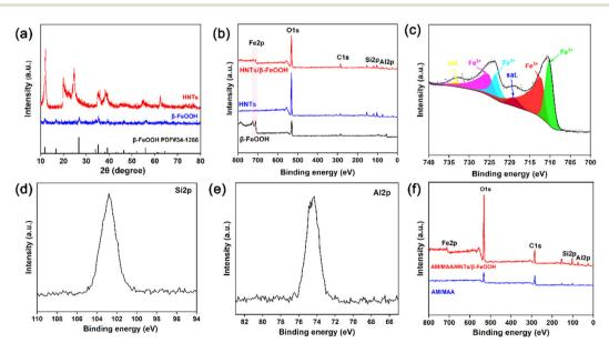
Fig. 2 (a) XRD diffraction patterns and (b) full XPS spectra of β-FeOOH, HNTs and HNTs/β-FeOOH. (c) XPS Fe 2p spectra of HNTs/β-FeOOH. XPS spectra of (d) Si 2p and (e) Al 2p of HNTs/ $\beta$ -FeOOH. (f) XPS full spectrum of AM/MAA/HNTs/ $\beta$ -FeOOH.
