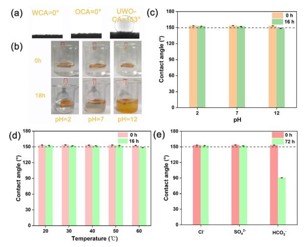
Fig. 3 (a) Oil contact angle of AM/MAA/HNTs/β-FeOOH sponge in air and underwater. (b) Photographs of the AM/MAA/HNTs/β-FeOOH sponge immersed in aqueous solutions of different pH. (c) Surface wettability of the sponge after immersion in solutions of different pH. Surface wettability of the AM/MAA/HNTs/β-FeOOH sponge after (d) immersion at different temperatures for 16 hours and (e) immersion in different ionic solutions (20 mM) for 72 hours.
