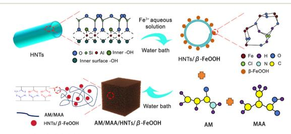
Fig. 1 Flow chart of AM/MAA/HNTs/β-FeOOH preparation.
