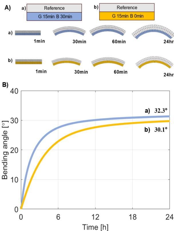
**Fig. 6** Computer simulation of 4D motions of hydrogel bi-layers of (a) **G15B30** + reference hydrogel and (b) **G15B0** + reference hydrogel in (A). (B) The simulated changes in the bending angles of the hydrogel bi-layer.
