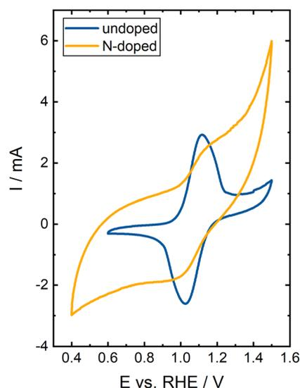
Fig. 8 CV of undoped and N-doped BC at a scan rate of 2 mV s<sup>-1</sup> in  $V(\text{IV})$  electrolyte.
