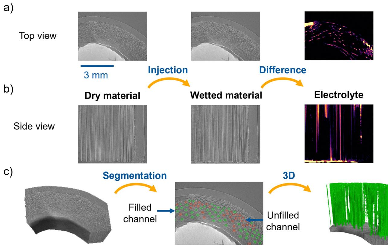
**Fig. 4** BC channel morphology and electrolyte filling: (a) 2D top and (b) side view of synchrotron X-ray tomograms conducted before (dry, left) and after (wet, center) electrolyte injection into a BC piece and corresponding images showing the difference between both tomograms (right); (c) 3D display of the respective tomogram (left) and the segmentation process (center; green: filled channel, red: unfilled channel) to achieve a 3D rendering of filled channels (right).
