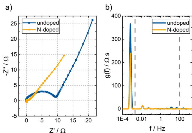
Fig. 7 (a) Nyquist plots and (b) DRT spectra of undoped and N-doped BC. A  $V(\text{IV})$  electrolyte and a flow rate of 15 mL min<sup>-1</sup> were used. A potential of 1.05 V vs. RHE was applied.
