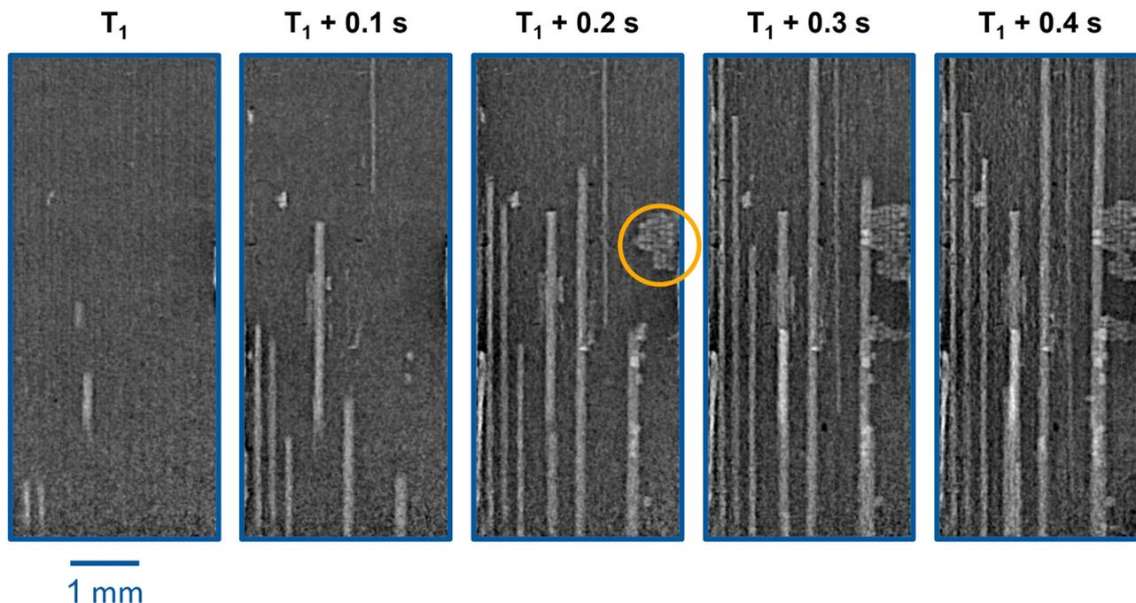
Fig. 5 Sequence of representative radiographs selected from synchrotron X-ray *in situ* 2D radiography experiment showing electrolyte injection in the BC tube.
