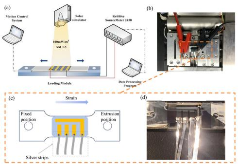
Fig. 1 Mechanical and electrical test of FPSCs. (a) Schematic diagram of the in-situ mechanical-photoelectrical testing platform; (b) the in situ tensile test apparatus; (c) and (d) the tensile testing sample of FPSCs prepared on a dog-bone shape flexible substrate.
