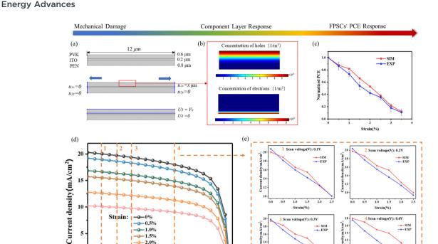
Fig. 4 (a) Two-dimensional geometric model and boundary conditions of the model; (b) the concentration distribution of electrons and holes in the perovskite layer; (c) the FPSCs' normalized PCE of experiment and simulation as a function of strain; (d) the simulated J-V curves of FPSCs under tensile strains from 0% to 2.5%; (e) the terminal current density as a function of the tensile strain under the scanning voltages of 0.1 V, 0.2 V, 0.3 V and 0.6 V.
