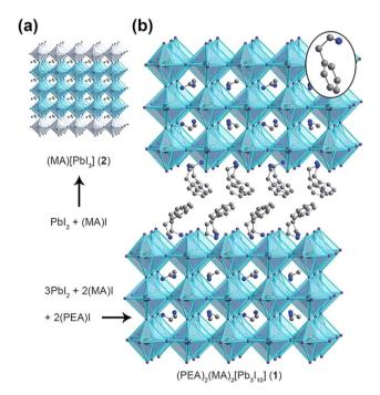
Fig. 6 Crystal structures of (a) 3D perovskite MAPbI and (b) 2D perovskite  $PEA_2MA_2Pb_3I_{10}$ . <sup>153</sup>
