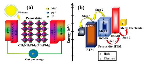
Fig. 2 (a) Working of PSCs and generation of electron-hole pairs in semiconductors, (b) energy levels in PSCs.<sup>36</sup>
