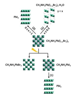
Fig. 5 Diagram of degradation of  $MAPb(I_{1-x}Br_x)_3$  exposed to humidity.<sup>151</sup>
