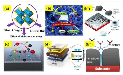
Fig. 4 (a) External factor effect on the stability of PSCs, (b-b") effect of water and moisture. Reproduced with permission.<sup>114</sup> Copyright 2015, American Chemical Society. (c) Influence of oxygen and (d) analysis of the heat effect.
