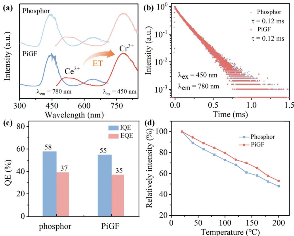
Fig. 3 (a) PL/PLE spectra ( $\lambda_{\text{ex}} = 450 \text{ nm}$ ;  $\lambda_{\text{em}} = 780 \text{ nm}$ ); (b) luminescence decay curves; and (c) QE and (d) temperature dependence of the integrated luminescence intensities of the CSSO:Ce,Cr,Li phosphor powders and the corresponding CSSO:Ce,Cr,Li PiGF-on-SP composite.
