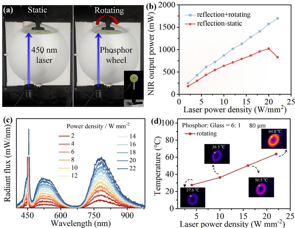
Fig. 5 (a) Digital photograph of the self-built laser system using a reflective light path and the fabricated phosphor wheel installed inside an integrating sphere. (b)  $P_{in}$ -dependent NIR output power of the optimal CSSO:Ce,Cr,Li PiGF-on-sapphire sample in static and rotating excitation modes. (c) EL spectra of the phosphor wheel when rotating under blue laser irradiation at different  $P_{in}$  values. (d) The  $P_{in}$ -dependent real-time temperature at the laser spot when rotating.
