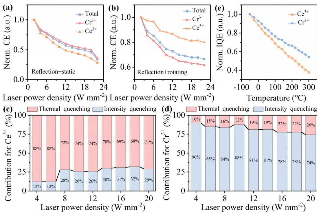
Fig. 6  $P_{in}$ -dependent relative conversion efficiencies of Ce<sup>3+</sup> and Cr<sup>3+</sup> in the PiGF sample in a reflective optical path in (a) static and (b) rotating excitation modes. The calculated contributions from thermal quenching and optical quenching for (c) Ce<sup>3+</sup> and (d) Cr<sup>3+</sup>. (e) The temperature-dependent relative IQEs for Ce<sup>3+</sup> and Cr<sup>3+</sup>.
