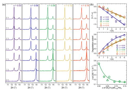
Fig. 6 (a) XRD results of  $GA_xFA_xMA_{1-2x}PbI_3$  compositions treated for various times at 200 °C. (b) Linear fits used to obtain the thermal degradation rate constants at 200 °C, experimental degradation extent data with reconstructed curves, and composition dependency of the rate constants.
