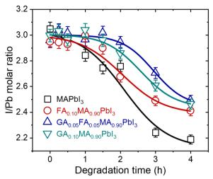
Fig. 3 Surface EDS iodine-to-lead molar ratio quantification as a function of time for samples treated at 200 °C. Lines were added as guides for the
