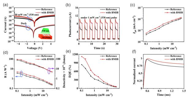
Fig. 3 (a) Dark and light I-V characteristics. (b) Current-time (I-t) characteristics of the reference and BMIB-based PDs. (c) Photocurrent density (J<sub>0t</sub>), (d) R (left axis), D\* (right axis), (e) EQE and (f) normalized transient photocurrent of the reference and BMIB-based PDs under green light at 2 V.
