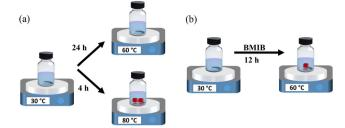
Fig. 1 Schematic of the crystallization procedure of the MAPbBr<sub>3</sub> SC (a) without and (b) with BMIB.
