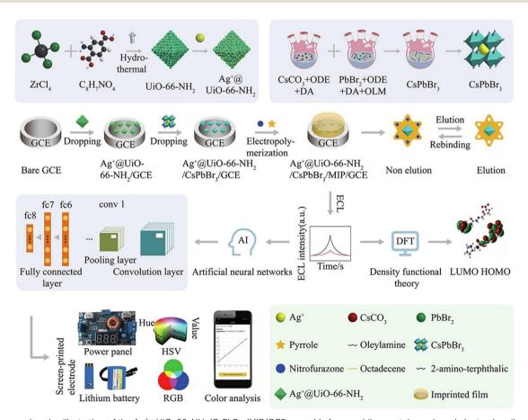
Fig. 4 A comprehensive illustration of the Ag+@UiO-66-NH2/CsPbBr3/MIP/GCE assembly for a mobile smartphone-based electrochemiluminescence molecularly imprinted polymer (ECL-MIP) system, depicting the intricate steps of preparation, integration of machine learning techniques, and the sensing mechanism. Adapted with permission. 123 Copyright 2022, Elsevier.
