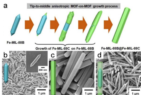
Fig. 4 (a) Schematic diagram of the apical to intermediate anisotropic MOF-on-MOF growth process. SEM images of (b) initial hexagonal rods of Fe-MIL-88B template, (c) pure Fe-MIL-88C hexagonal rods, and (d) Fe-MIL-88B@Fe-MIL-88C core–shell hybrid hexagonal rods. (Panels a–d) Reproduced with permission. 18 Copyright 2020, American Chemical Society.
