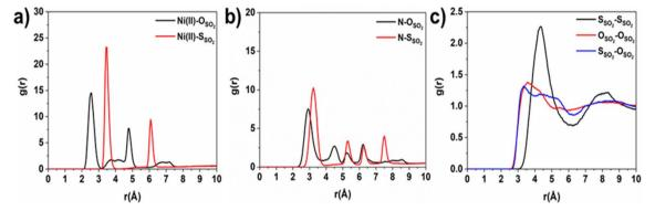
Fig. 6 Intermolecular radial pair distribution functions of NiBDP-0H<sub>2</sub>O MOF atoms and adsorbed  $SO_2$  molecules were calculated at P = 0.10 bar (a and b), and guest  $SO_2-SO_2$  (c) was calculated at P = 0.50 bar.
