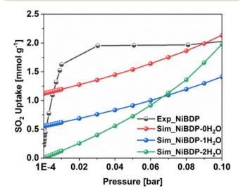
Fig. 4 Comparison of SO<sub>2</sub> adsorption isotherms in NiBDP MOFs, obtained experimentally and calculated by GCMC simulations at 298 K for 3 different structure models containing 0, 1 or 2 water molecules per unit cell, covering a pressure range from  $1 \times 10^{-4}$  to 1 bar.
