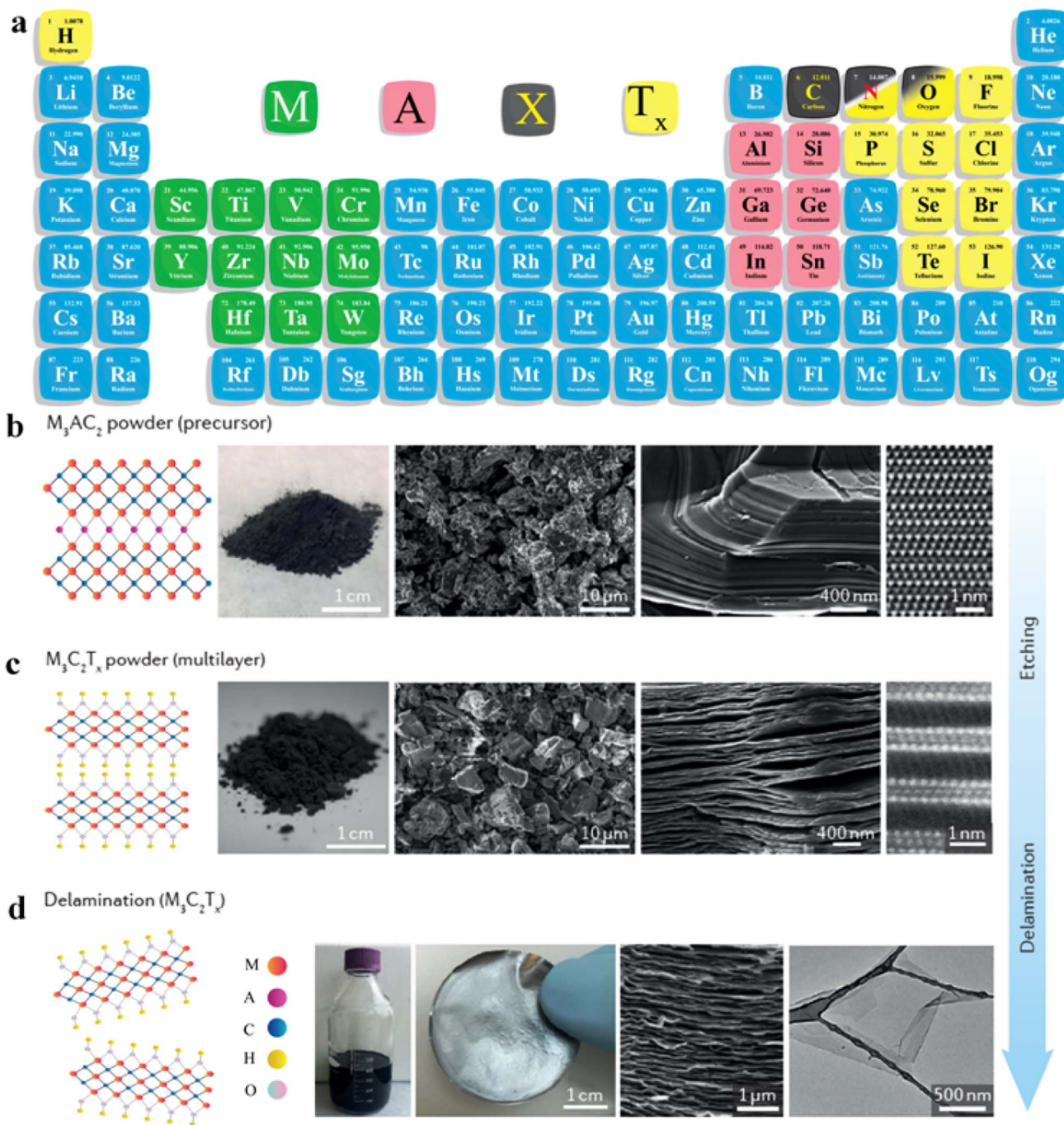
Fig. 1 (a) Important elemental constituents of MAX and MXenes. The black highlight in O represents oxycarbides and oxynitrides, reproduced from ref. 11 with permission from Royal Society of Chemistry, copyright 2022. (b and c) Atomic structure, SEM and HR-STEM results of precursors of MAX ( Ti_3AlC_2 ) and a multi-layered MXene ( M_2C_2T_x ). (d) SEM image of a Mo_2TiC_2T_x film of Ti_3C_2T_x in water along with a digital view and TEM image of Ti_3C_2T_x flakes, reproduced from ref. 60 with permission from Nature Reviews Materials , copyright 2017.
