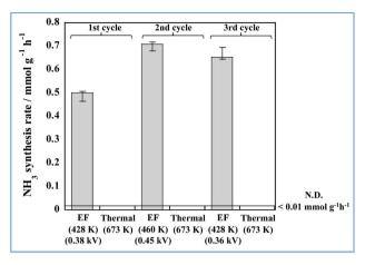
Fig. 6 Cyclic results obtained for thermal catalysis and catalytic reactions in an electric field (denoted as EF).
