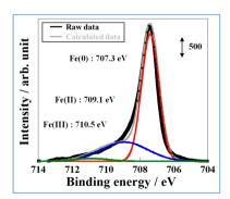
Fig. 4 Fe 2p X-ray photoelectron spectra of FeP.
