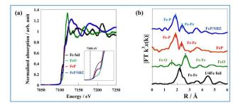
Fig. 3 (a) Fe K-edge XANES spectra of the Fe foil, FeO, FeP, and FeP/ SBZO, and (b) Fourier transformation of the  $k^3$ -weighted EXAFS of the Fe foil, FeO, FeP, and FeP/SBZO.
