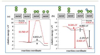
Fig. 9 Energy diagram of N<sub>2</sub> dissociation (a) and N<sub>2</sub>H formation (b) on Fe(110) and FeP(31-1). Activation energy for N2 dissociation in the absence of an electric field corresponds to the energy difference between the second state and the third state in (a). N<sub>2</sub>H production energy in an electric field corresponds to the energy difference between the second state and the fourth state in (b).
