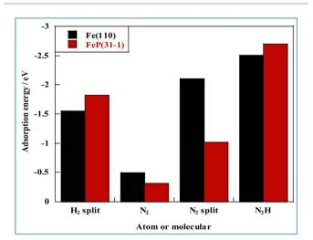
Fig. 7 Molecular and atomic adsorption energies related to NH<sub>3</sub> synthesis for different metal species.
