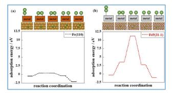
Fig. 8 Intermediate states of N<sub>2</sub> dissociation calculated using the NEB method. Energy diagram of N<sub>2</sub> dissociation calculated using the NEB method: (a) Fe(110) and (b) FeP(31-1), where purple, brown, and green balls respectively represent P, Fe, and N. Because the second coordination (the first intermediate state) is the most unstable on both surface models, its energies were adopted as the energies of transition
