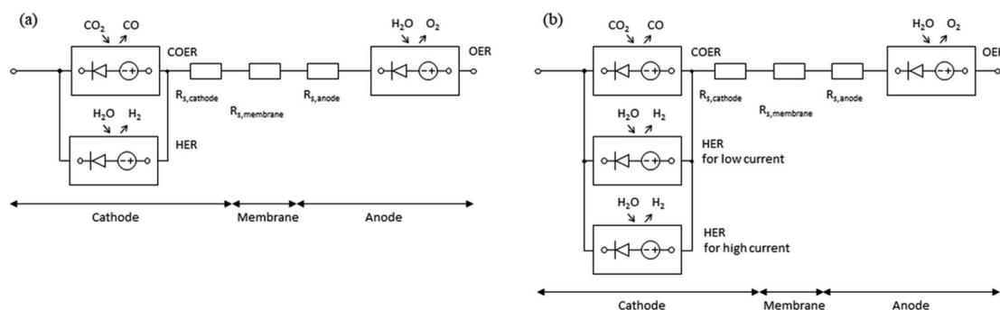
Fig. 2 Equivalent circuit models for  $\text{CO}_2$  EC. (a) Equivalent circuit of the cathode with a parallel connection between a COER element and one HER element. (b) Equivalent circuit of the cathode with a parallel connection between a COER element and two HER elements (low current density and high current density).
