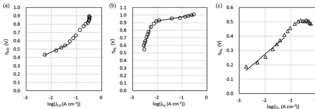
Fig. 5 Tafel plots at a CO<sub>2</sub> flow rate of 5 sccm cm<sup>-2</sup> and cell temperature of 50 °C. (a) CO evolution reaction (COER). (b) H<sub>2</sub> evolution reaction (HER). (c) O<sub>2</sub> evolution reaction (OER).
