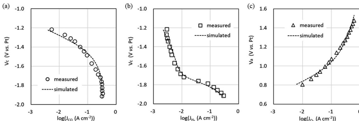
Fig. 6 Measured cathode potential  $V_c$  and anode potential  $V_a$  relative to the Pt pseudo-reference electrode and simulation using the equivalent circuit model in Fig. 2b. (a) CO evolution reaction (COER). (b)  $H_2$  evolution reaction (HER). (c)  $O_2$  evolution reaction (OER).
