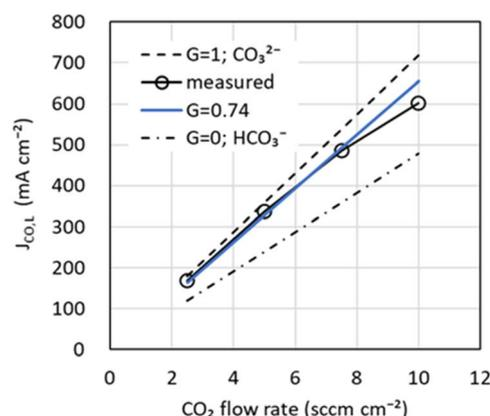
Fig. 4 CO limiting current density versus CO<sub>2</sub> flow rate input from the cathode channel. Markers are experimental values. Dotted, dotted-dashed, and solid blue lines are calculated values for  $G = 1$  (CO<sub>3</sub><sup>2-</sup>),  $G = 0$  (HCO<sub>3</sub><sup>-</sup>), and  $G = 0.74$  (CO<sub>3</sub><sup>2-</sup>; 74%, HCO<sub>3</sub><sup>-</sup>; 26%), respectively.  $G$  is the fraction of CO<sub>3</sub><sup>2-</sup> that transfers from the cathode to the anode.
