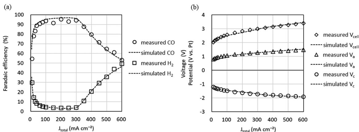
Fig. 7  $CO_2$  EC performance versus total current density ( $J_{total}$ ). (a) faradaic efficiencies of CO and  $H_2$ . (b) Cell voltage ( $V_{cell}$ ), anode potential ( $V_a$ ), and cathode potential ( $V_c$ ) ( $CO_2$  flow rate, 5 sccm  $cm^{-2}$ ; cell temperature, 50 °C). Markers show measured values and dotted lines show simulated values.
