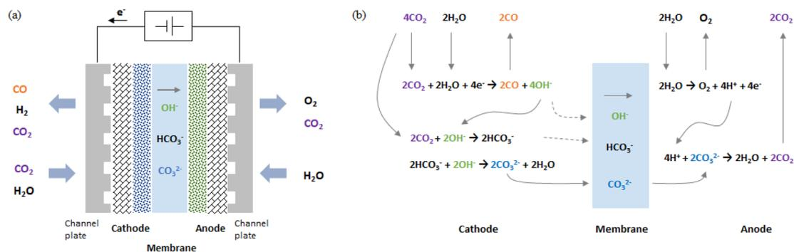
Fig. 1 Schematic drawing of (a) configuration of zero-gap type CO<sub>2</sub> EC producing CO and (b) electrochemical and chemical equilibrium reaction steps.
