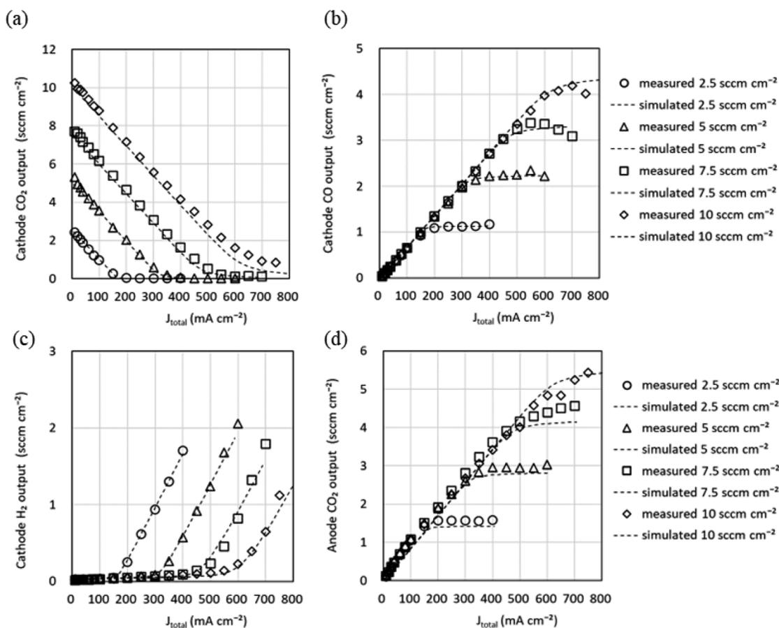
**Fig. 8** Gas flow rate output from the cathode and anode channels versus total current density ( $J_{total}$ ) for four CO<sub>2</sub> input flow conditions. (a) CO<sub>2</sub>, (b) CO, and (c) H<sub>2</sub> are output from the cathode channel. (d) O<sub>2</sub> is output from the anode channel. Experimental data are shown as markers and simulation data using the values listed in Tables 2 and 3 and  $G = 0.74$  as dotted lines.
