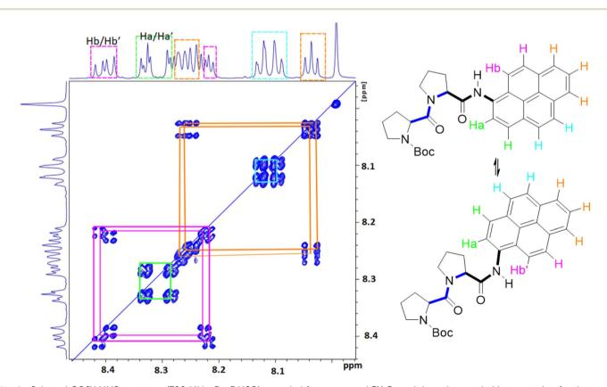
Fig. 2 Selected COSY NMR spectrum (700 MHz,  $D_6$ -DMSO) recorded for compound PY-P<sub>2</sub> and the colour coded interpretation for the two isomers.
