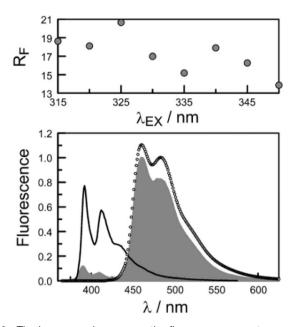
**Fig. 9** The lower panel compares the fluorescence spectrum recorded for  $PY-P_8-PER$  in chloroform (shaded profile) following excitation at 350 nm with spectra projected for  $P_{EET}$  values of 0% (black curve) and 100% (open circles). The upper panel illustrates how the ratio of integrated emission profiles depends on excitation wavelength.
