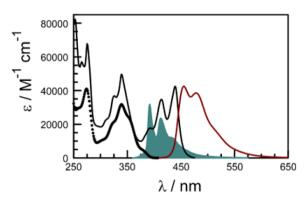
Fig. 7 Absorption (black curve) and fluorescence (brown curve) spectra recorded for  $PY-P_8-PER$  in  $CHCl_3$  at room temperature. The excitation wavelength was 420 nm. The open circles indicate the absorption spectrum for the pyrene component extracted by global curve fitting routines while the solid blue curve shows the normalised fluorescence spectrum for the pyrene emitter to indicate the good spectral overlap.
