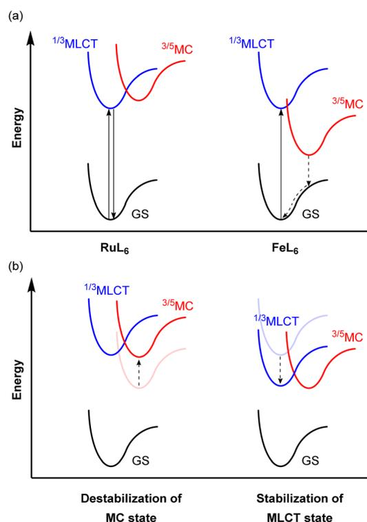
Fig. 21 (a) Simplified potential energy surface diagrams of six-coordinate  $\text{Ru}(\text{II})$  and  $\text{Fe}(\text{II})$  complexes. (b) Strategies to achieve a larger energy barrier between MLCT and MC states.
