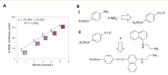
Fig. 6 Detection of nitrate in the proposed μPAD. (A) Calibration curve obtained for ammonium in concentrations ranging from 0.5 to 10.0 mmol L<sup>-1</sup>. (B) Reaction between (i) nitrite and sulfanilamide, forming a diazo compound; (ii) diazo compound and NED, forming an azo dye with a redpurple color, allowing the quantification of nitrate.
