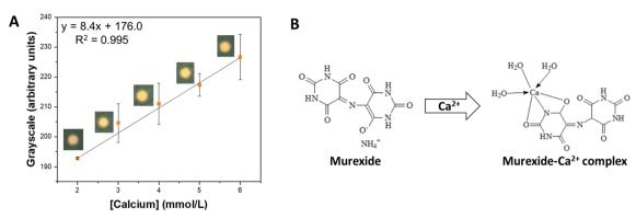
Fig. 3 Detection of calcium in the proposed  $\mu$ PAD. (A) Calibration curve obtained for Ca<sup>2+</sup> in concentrations ranging from 2.0 to 6.0 mmol L<sup>-1</sup>. (B) Structure of murexide and the murexide–Ca<sup>2+</sup> complex.
