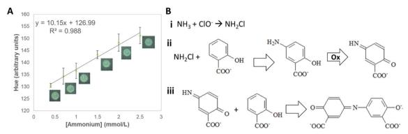
Fig. 5 Detection of ammonium in the proposed μPAD. (A) Calibration curve obtained for ammonium in concentrations ranging from 0.5 to  $2.5 \text{ mmol L}^{-1}$ . (B) Reaction between (i) ammonium and hypochlorite, forming monochloramine; (ii) monochloroamine and salicylate, forming 5aminosalicylate and (iii) 5-aminosalicylate being oxidized in the presence of nitroprusside catalyst forming the blue colored indosalicylate
