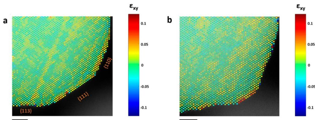
Fig. 5 Strain analysis of a PtCu<sub>3</sub> nanoparticle. Shear strain ( $\epsilon_{xy}$ ) map (a) before and (b) after electrochemical activation.<sup>60</sup> Open access, 2019.
