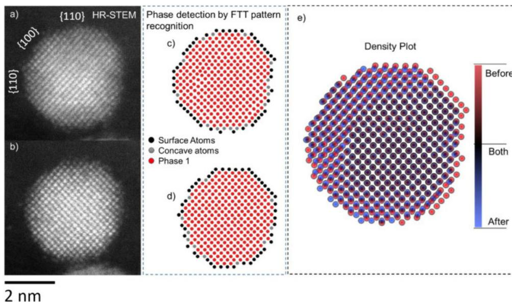
**Fig. 9** IL-STEM images of a Pt–Co nanoparticle (a) before and (b) after electrochemical activation. Atomic positions obtained *via* phase detection using FFT patterns, (c) before and (d) after activation. (e) Density plot of atomic positions before and after, overlaid.<sup>98</sup> Open access, 2021.
