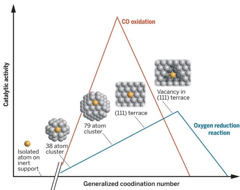
**Fig. 1** Dependence of Pt catalytic activity for ORR and CO oxidation on the generalized coordination number. The coordination of the active site has a clear impact on the performance of the catalyst. Reproduced with permission ref. 33. Copyright 2015, AAAS.
