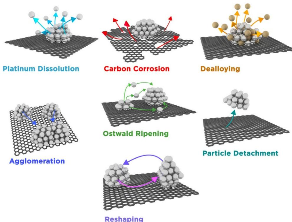
Fig. 6 An illustration of different degradation mechanisms of Pt nanoparticles supported by carbon.<sup>83</sup> Open access, 2016.
