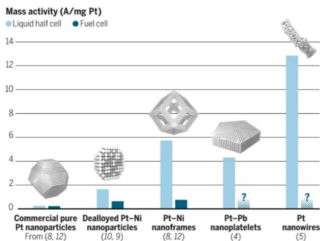
**Fig. 4** A comparison of ORR mass activity of different Pt and Pt-based catalyst nanostructures. The activities of more intricate nanostructures exceptionally decrease when comparing an experimental half cell to MEA, indicating that additional challenges arise in real fuel cell implementation. Reproduced with permission ref. 48. Copyright 2016, AAAS.
