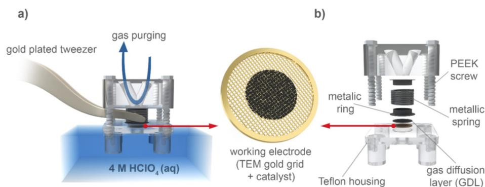
**Fig. 8** An illustration of the modified floating electrode (MFE) setup.<sup>97</sup> Open access, 2020.
