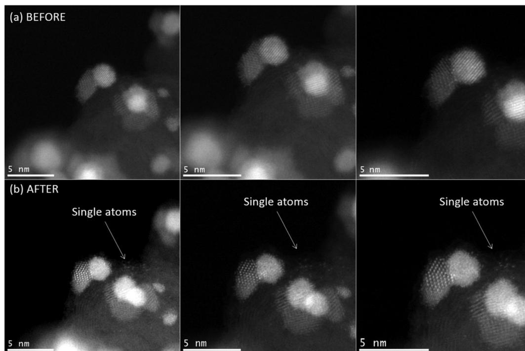
**Fig. 7** IL-STEM images of Pt-SnO<sub>2</sub>/C nanoparticles (a) before and (b) after 1000 electrochemical cycles from 0.05–9.8 V (vs. RHE) at different magnifications. Single atoms appear after degradation and are shown to not move from beam exposure. Reprinted with permission from *J. Phys. Chem. C*, 2018, **122**(18), 10050–10058.<sup>96</sup> Copyright 2018, American Chemical Society.
