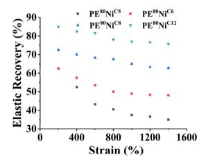
Fig. 10 Elastic recovery percentages of PE samples generated at 80 °C by catalysts  $Ni^{C5}$ ,  $Ni^{C6}$ ,  $Ni^{C8}$ , and  $Ni^{C12}$ .
