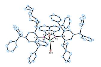
Fig. 5 Molecular structure of Ni<sup>C12</sup> with thermal ellipsoids shown at a 30% probability level. All hydrogen atoms are omitted for clarity. Selected bond lengths (Å): Ni1–Br1 2.327(12), Ni1–Br2 2.318(11), Ni1–N1 2.015(5), Ni1–N2 2.040(5), C1–C2 1.509(8), N1–C1 1.281(8), N2–C2 1.270(8), N1–C4 1.453(7), N2–C3 1.456(7); and bond angles (°): Br1–Ni1–Br2 121.39(5), N1–Ni1–N2 83.2(2), N1–Ni1–Br1 110.31(14), N1–Ni1–Br2 113.12(14), N2–Ni1–Br1 113.70(15), N2–Ni1–Br2 108.81(14).
