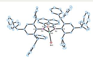
Fig. 3 Molecular structure of Ni<sup>C5</sup> with thermal ellipsoids shown at a 30% probability level. All hydrogen atoms are omitted for clarity. Selected bond lengths (Å): Ni1–Br1 2.334(6), Ni1–Br2 2.331(6), Ni1–N1 2.035(2), Ni1–N2 2.042(2), C1–C2 1.513(3), N1–C1 1.282(3), N2–C2 1.281 (4), N1–C4 1.441(3) N2–C3 1.450(3); and bond angles (°): Br1–Ni1–Br2 124.09(3), N1–Ni1–N2 83.28(9), N1–Ni1–Br1 115.83(6), N1–Ni1–Br2 103.74(6), N2–Ni1–Br1 106.72(6), N2–Ni1–Br2 116.04(7).
