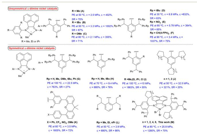
Fig. 1 Structural modifications in  $\alpha$ -diimine nickel precatalysts and their impact on the mechanical and elastic properties (data reported of mechanical and elastic properties herein is selected for those polyethylene samples which were prepared at the highest reaction temperature).
