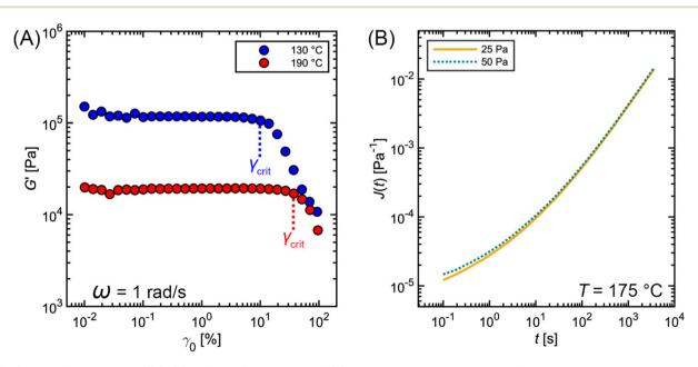
Fig. 11 Commercial polystyrene (A) SAOS strain amplitude sweep and (B) creep measurements at varying shear stress.
