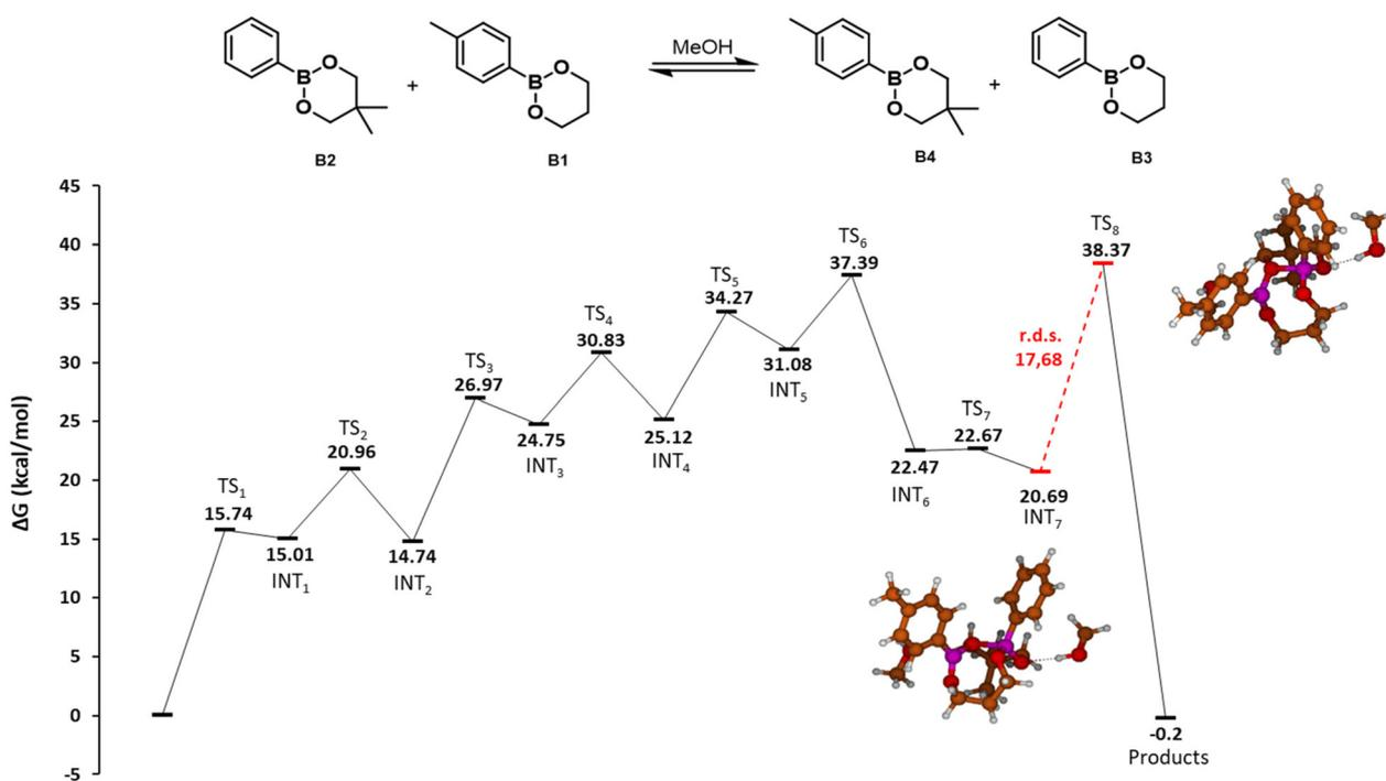
**Fig. 2** Potential energy surface of the MeOH-mediated exchange of dioxaborinanes. Gibbs free energies ( $\Delta G$ ) in  $\text{kcal mol}^{-1}$ . Red line indicates the r.d.s. of the reaction with the value in  $\text{kcal mol}^{-1}$ . The molecular structures corresponding to the intermediates and transition states are depicted in the ESI.†
