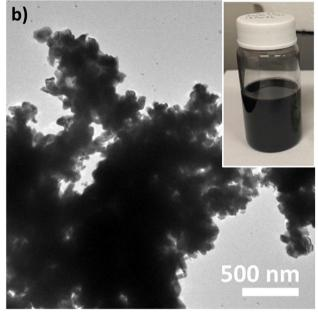
Fig. 1 (a) PXRD of the obtained black  $ln_2O_{3-x}$  compared to the simulated pattern for bixbyite  $In_2O_3$ . (b) TEM image of the black  $In_2O_{3-x}$ showing dense agglomerations. The inset shows a picture of the particles dispersed in toluene.
