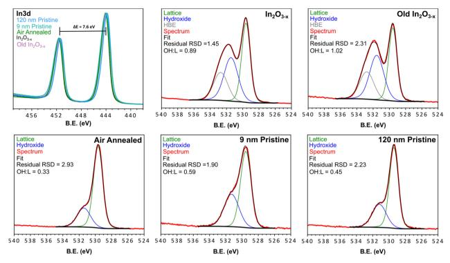
Fig. 6 XPS spectra of the black  $In_2O_{3-x}$ , aged black  $In_2O_{3-x}$ , air annealed, 9 nm pristine, 120 nm pristine, and commercial samples. Each spectrum was fit with lattice and surface hydroxyl groups, while the black  $In_2O_{3-x}$  samples displayed an additional HBE feature. The Survey scans of each material are found in Fig. S24† and peak fitting parameters for the O 1s fitting are found in Table S3.†
