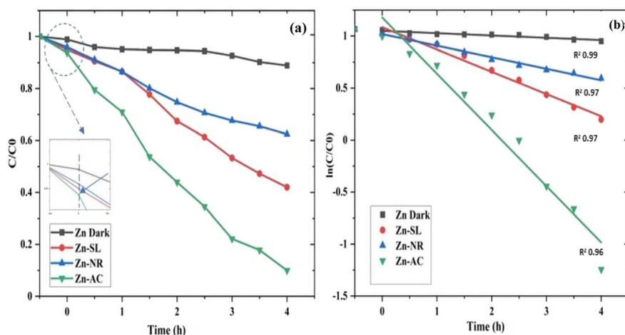
Fig. 11 (a and b) A concentration ( $C/C_0$ ) vs. time plot (a) showing decrease in dye concentration with time for different catalyst systems and (b) a plot of ( $\ln C/C_0$ ) vs. time showing pseudo-first-order kinetics with slope (rate constant " $k$ ") in  $m = -0.04161$  to  $-0.07473$  with  $R^2$  values in the range of 0.95 to 0.99.
