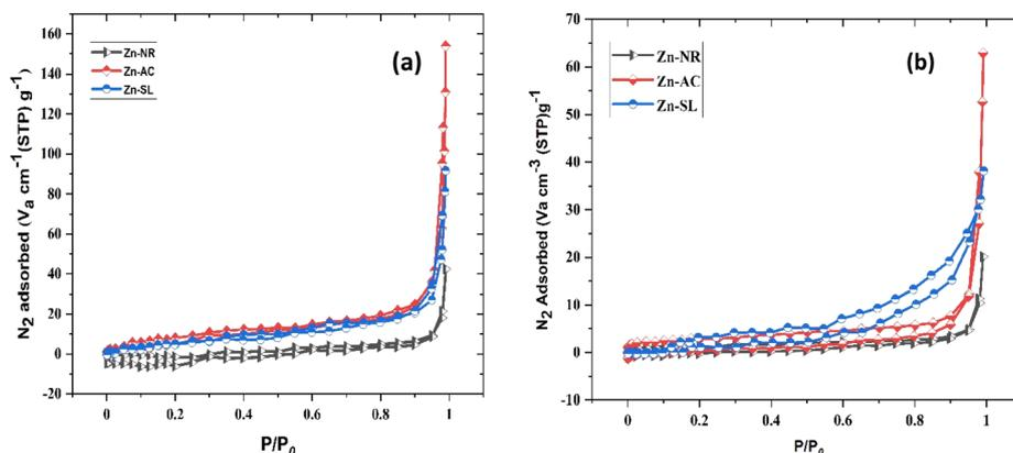
Fig. 16 (a) N<sub>2</sub> adsorption–desorption isotherm of the three catalysts used (Zn-AC, Zn-SL, and Zn-NR), indicating the changes in the surface area of the catalysts (pre- and post-use) by Brunauer–Emmett–Teller (BET) analysis (before use) and (b) isotherm curves after the use of the catalysts.
