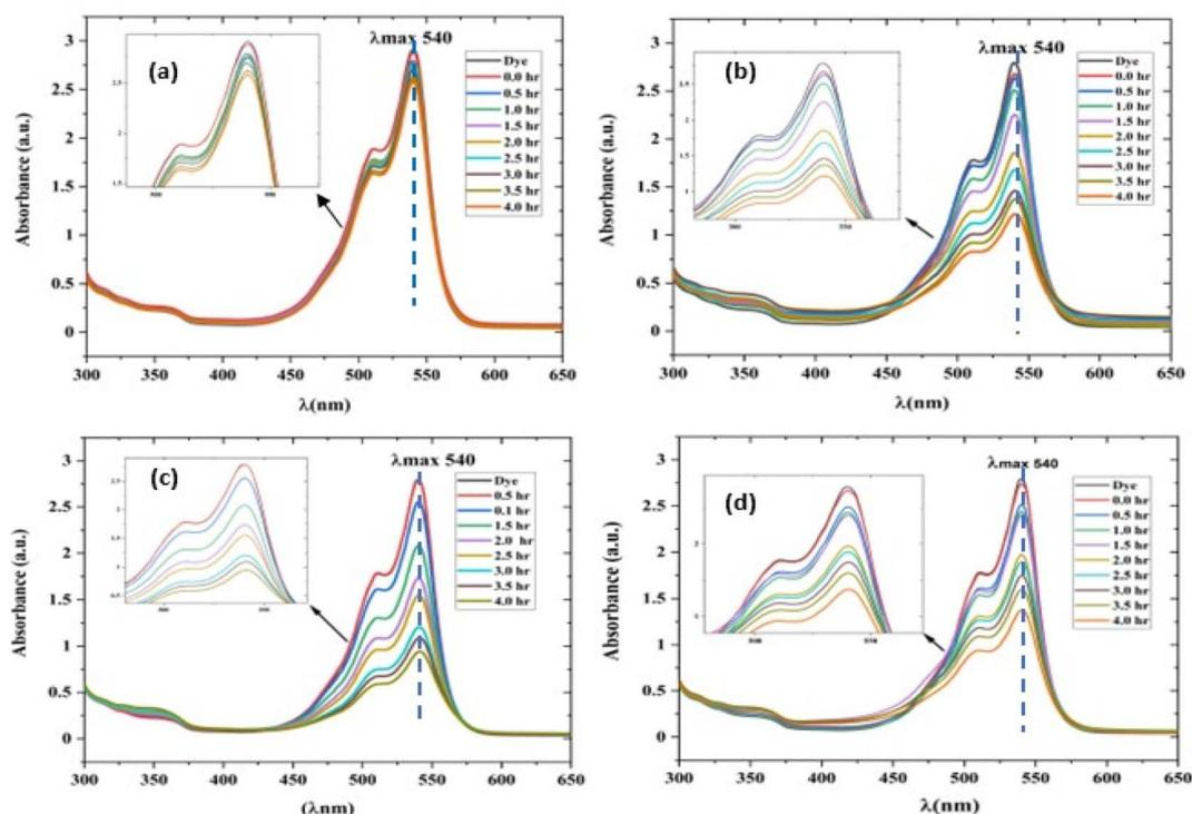
Fig. 10 UV-visible absorption spectrum of a rhodamine dye (conc.  $0.596 \times 10^{-3}$ ) and photocatalyst (conc.  $100 \text{ mg L}^{-1}$ ) suspension system under exposure to direct sunlight recorded at the time interval of 0.5 h. (a) The control experiment (dye-catalyst system in the dark) and (b) Zn-SL, (c) Zn-AC and (d) Zn-NR catalyst systems.
