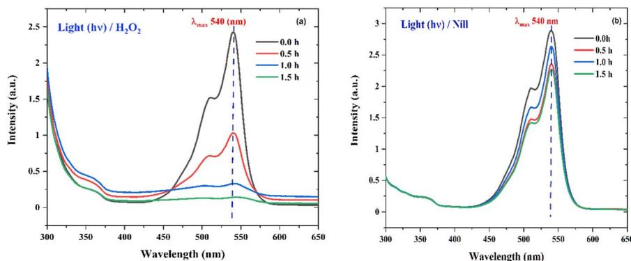
Fig. 15 (a) The UV absorption degradation curves of RhB dye with Zn-AC catalyst suspension system for the hydrogen peroxide (H<sub>2</sub>O<sub>2</sub>) experiment in the presence of light (*hν*). (b) The UV absorption degradation curve of RhB dye with Zn-AC catalyst suspension system for hydrogen peroxide (H<sub>2</sub>O<sub>2</sub>) control experiment (without H<sub>2</sub>O<sub>2</sub> in the presence of light (*hν*)).
