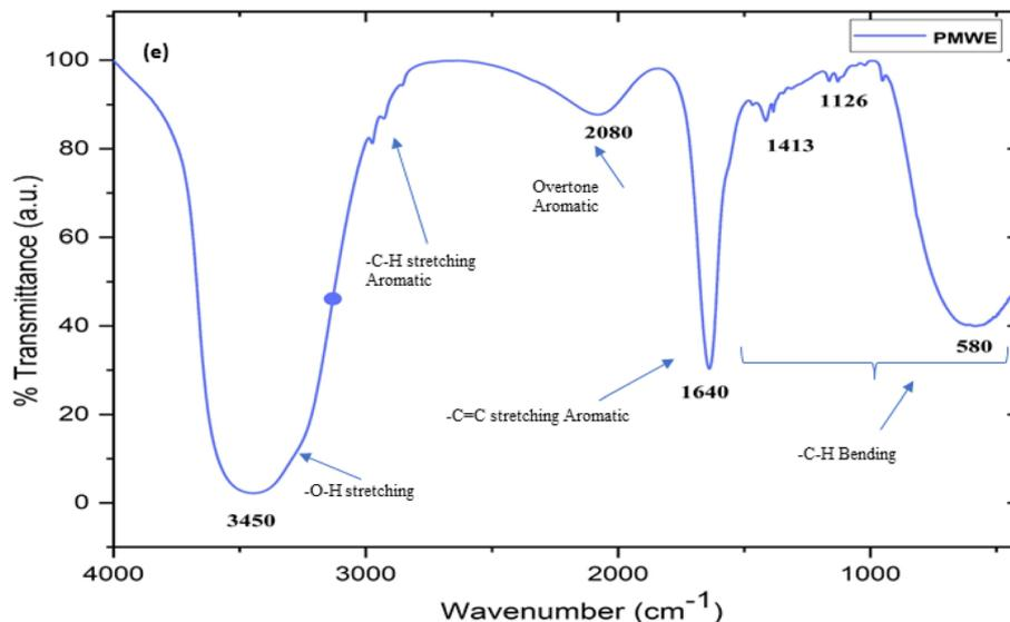
Fig. 17 The Fourier-transform infrared spectrum (FTIR) of sugarcane press mud water extract (PMWE) with characteristic stretching peaks corresponding to the functional groups of the analyte present in the sample.
