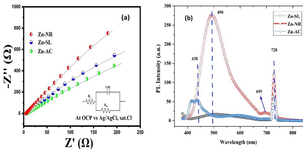
Fig. 13 (a) The electrochemical impedance spectra of the Zn-AC, Zn-SL, and Zn-NR catalysts showing different charge transfer resistance ( $R_{ct}$ ) at the electrode/electrolyte interface. (b) The photoluminescence spectra of the same catalysts showing their ( $e^-$ ) and ( $h^+$ ) pair recombination behaviour.
