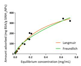
Fig. 3 Adsorption isotherms of BSA over SiOHNPs (A) and SiNH<sub>2</sub>NPs (B) with representation of Langmuir and Freundlich curves in orange and green, respectively
