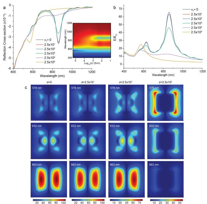
Fig. 2 Simulated quantum correction model metasurface: (a) simulated reflectance spectra for metasurface with constant gap height (2 nm) and varied conductivity  $\sigma_T$ , insert is reflectance intensity map for metasurface with different conductivity (b) simulated average electric field enhancements for metasurface with constant gap height (2 nm) and varied conductivity  $\sigma_T$ . (c) Near-field distribution for metasurface with different conductivity  $\sigma_T$
