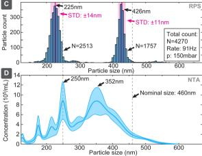
distribution and concentration measurement polydisperse samples represented by mixture of 252 nm and 460 nm particles in respective concentrations of  $5.7 \times 10^9$  and  $2.9 \times 10^9$ particles per mL. (A) Raw measured signal (blue) with detected particles indicated with red. (B) Same in enlarged scale. (C) Histograms of populations of spikes corresponding to both sizes of particles, while (D) shows NTA measurement of mixture of same particles (108 particles per mL each).
