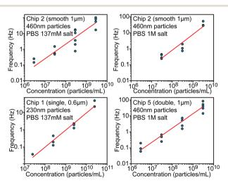
**Fig. 5** Evaluation of particle concentration. Relationship between the particle concentration and spiking frequency shown in log-log scale.
