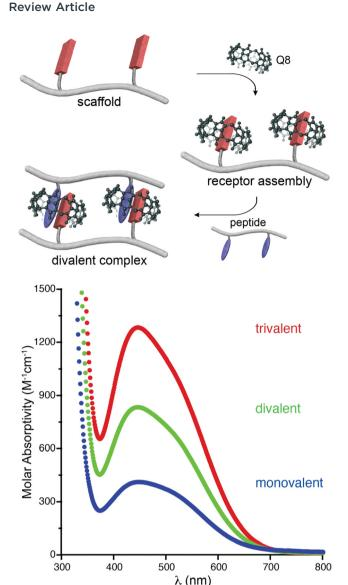
Fig. 7 (top) Schematic of the self-assembly of Q8 onto a divalent scaffold and the divalent binding of the resulting receptor to a divalent peptide. (bottom) UV-visible spectra showing the additive molar absorptivities of monovalent, divalent, and trivalent complexes. 47 Reproduced with permission from ref. 47. Copyright 2009 American Chemical Society.
