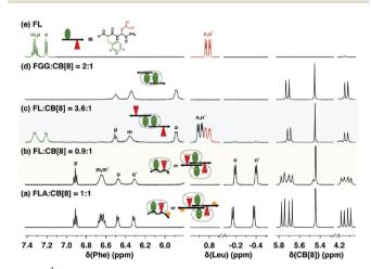
Fig. 13 <sup>1</sup>H NMR spectra of H-Phe-Leu-Ala-NH<sub>2</sub> (FLA) and H-Phe-Leu-NH<sub>2</sub> (FL) at various ratios with Q8, showing patterns of signal perturbation that indicate the binding modes shown schematically. CB[8] is Q8.51 Reproduced from ref. 51 with permission from the Royal Society of Chemistry
