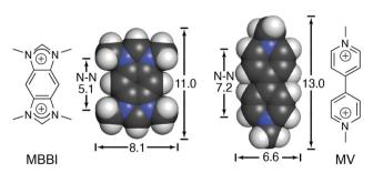
Fig. 10 Chemical formulas and space-filling models of MBBI and MV, showing size comparisons in Angstroms.<sup>59</sup> Reproduced with permission from ref. 59. © 2010 Wiley-VCH Verlag GmbH & Co. KGaA, Weinheim.
