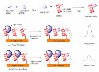
Fig. 22 Protein sensing technique through electrochemical readout at a gold surface. CB[8] is Q8. 109 Reproduced with permission from ref. 109. Copyright 2012 American Chemical Society.
