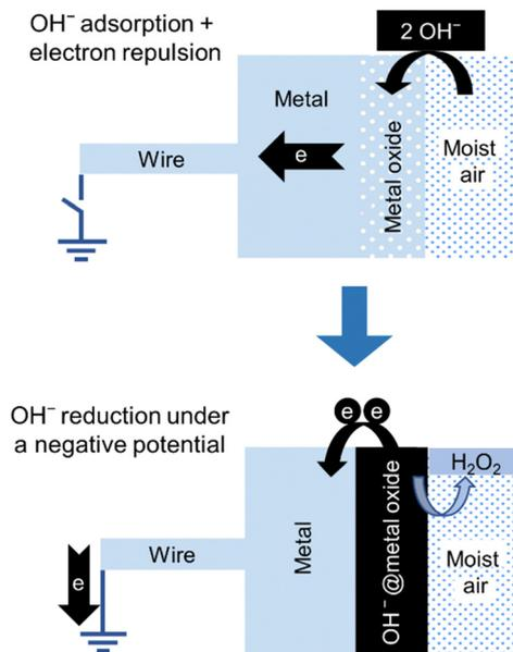
**Fig. 15** Stepwise description of the two steps in the negative electrode of a hygroelectric cell: (top) adsorption: an isolated electroneutral acidic oxide surface in contact with moisture adsorbs  $\text{OH}^-$  ions acquiring negative charge. (bottom) Redox reaction: electron transfer from  $\text{OH}^-$  ions to the electrode produces hydrogen peroxide. Adapted with permission from ref. 131. Copyright 2023. American Chemical Society.
