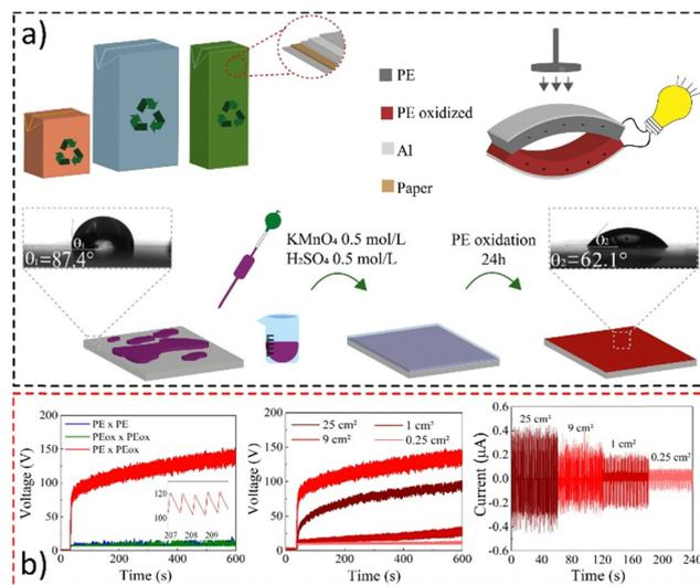
**Fig. 20** (a) Fabrication of a simple triboelectric energy harvesting device using a laminated food packaging film. LDPE surface oxidation with  $\text{KMnO}_4$  solution lowered the water contact angle. (b) Open-circuit voltage using different dielectric-to-dielectric pairs and the (d) open-circuit voltage and (e) short-circuit current on samples with different sizes. Adapted from ref. 192, Copyright (2023), with permission from Elsevier.
