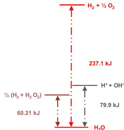
Fig. 13 Diagram showing the standard Gibbs energy levels for water, hydrogen peroxide, the ions formed by water self-ionization, and H<sub>2</sub> + ½O<sub>2</sub>. Reprinted with permission from ref. 131. Copyright 2023. American Chemical Society.
