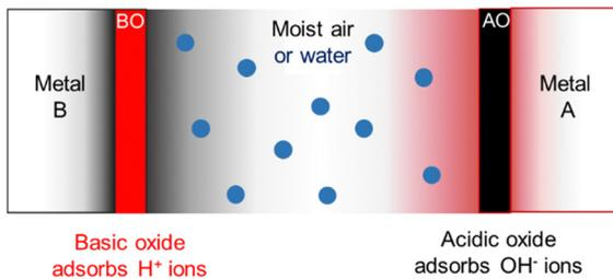
**Fig. 14** Electrified compartments in a hygroelectric cell made from parallel plates of conductive materials, metals A and B. The oxide AO adsorbs  $\text{OH}^-$  ions becoming negative and repelling negative charge in the supporting metal, while BO becomes positive by adsorbing  $\text{H}^+$  ions. Excess charge in the oxides produces a potential difference between metals A and B. Adapted with permission from ref. 131. Copyright 2023. American Chemical Society.
