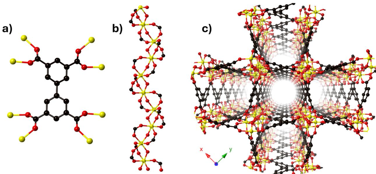
**Fig. 1** MFM-300(M) (M = Sc(III), Al(III), In(III), Cr(III), V(III), Ga(III) and Fe(III)) ligand-metal framework structure constitution. (a) Coordination arrangement of BPTC<sup>4-</sup> ligand (C atoms in grey, O atoms in red, hexacoordinated metal ions in yellow (Sc, In)); (b) M(OH)(CO<sub>2</sub>)<sub>2</sub>, 1D chiral chain; (c) MFM-300(Sc, In) cylindrical channels viewed along the c axis.
