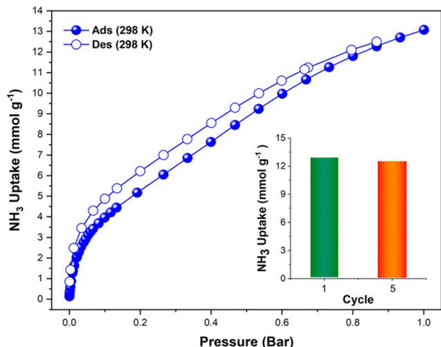
**Fig. 2** Experimental  $\text{NH}_3$  adsorption–desorption isotherms of MFM-300(Sc) (filled blue circles = adsorption; open blue circles = desorption) at 298 K and up to 1 bar. Inset: comparison of  $\text{NH}_3$  uptake of MFM-300(Sc) from the first and fifth adsorption cycles (13.1 and 12.6  $\text{mmol g}^{-1}$ , respectively, 3.8% decrease) at 298 K and up to 1 bar. Reproduced with permission from ref. 26. Copyright 2021, American Chemical Society.
