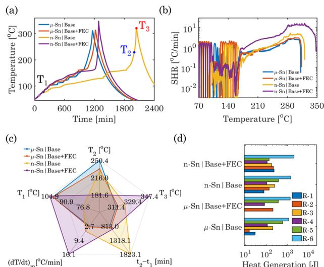
**Fig. 2** The ARC experiments to probe the thermal stability of the Sn electrode. (a) Temperature response of  $\mu$ -Sn and n-Sn-based half-cell using the electrolytes—base and base + FEC. (b) The temperature increase and the corresponding self-heating rates (SHR) for all the cases. (c) Thermal safety characteristics and (d) comparison of heat generation of the  $\mu$  and n-Sn cases in two different electrolytes.
