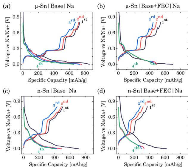
**Fig. 1** Voltage profile of  $\mu$ -Sn based half-cell using the electrolytes of (a) EC:PC:DEC-base, (b) EC:PC:DEC:FEC-base + FEC, and n-Sn-based half-cell using the electrolytes of (c) EC:PC:DEC-base, (d) EC:PC:DEC:FEC-base + FEC.
