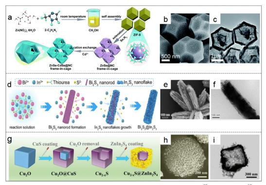
Fig. 4 Illustration of the preparation processes and micrographs of (a–c) ZnSe–CdSe@NC frame-in-cage,  $^{59}$  (d–f) Bi<sub>2</sub>S<sub>3</sub>@In<sub>2</sub>S<sub>3</sub>, $^{60}$  and (g–i) Cu<sub>2-x</sub>S@Z-nIn<sub>2</sub>S<sub>4</sub> core–shell hollow nanoboxes.  $^{61}$
