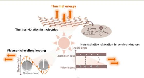
Fig. 2 Different mechanisms of photo-to-thermal process in various materials. 18
