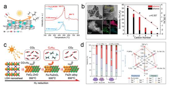
Fig. 8 (a) Scheme and CO adsorption ability of  $Fe_5C_2/NC600.75$  (b) Characterization data and product selectivity of the Ni/MnO catalyst. (c) The CO hydrogenation selectivities of the Fe-x photocatalysts derived from ZnFeAl-LDH nanosheets at different temperatures.<sup>77</sup> (d) Comparison of FTS performance of Ru<sub>1</sub>Co-SAA with other catalysts. 80
