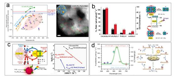
Fig. 9 (a) WGS performance and morphology of the  $Pt/\alpha$ -MoC catalyst. 83 (b) WGS activity and mechanism of the  $CuO_x/Al_2O_3$  catalyst. 86 (c) WGS reaction mechanism and the apparent activation energy of the  $CeO_2/Cu_{1.5}Mn_{1.5}O_4$  catalyst. 87 (d) WGS reaction activity and mechanism of the LD-Cu catalyst. 96
