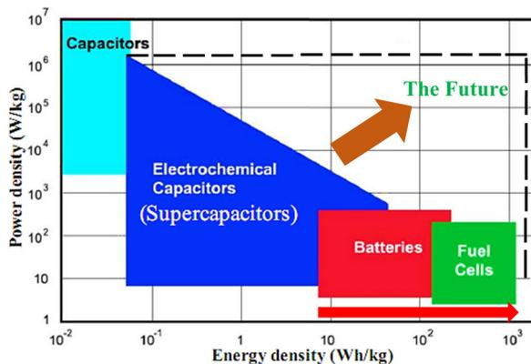
Fig. 2 Illustration of the variation in energy density and power density of various electrochemical energy storage systems and envisaged future research direction and development for electrochemical energy storage systems.
