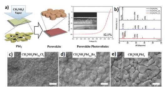
Fig. 11 (a) Schematic illustration of perovskite film formation through a vapor-assisted solution process. Adapted with permission from ref. 147. (b) XRD patterns for films of  $CH_3NH_3PbI_3$ ,  $CH_3NH_3PbI_{3-x}Br_x$ , and  $CH_3NH_3PbI_{3-x}Cl_x$  deposited by the VASP method. FTO = fluorine-doped tin oxide. SEM surface images of (c)  $CH_3NH_3PbI_3$ , (d)  $CH_3NH_3PbI_3$ , and (e)  $CH_3NH_3PbI_3$  deposited by the VASP method. Scale bars are 500 nm. Adapted with permission from ref. 148.
