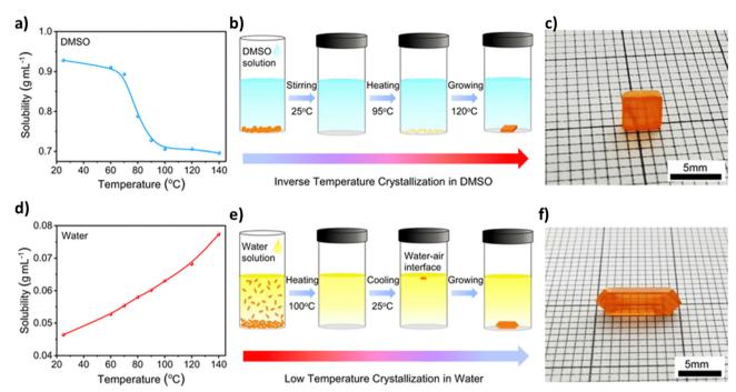
Fig. 16 (a) Temperature-dependent solubility of CsPbBr<sub>3</sub> in DMSO. (b) Schematic illustration of the inverse-temperature crystallization in DMSO (c) Optical image of the as-prepared CsPbBr<sub>3</sub> SC. (d) Temperature-dependent solubility of CsPbBr<sub>3</sub> in water. (e) Schematic illustration of the lowtemperature crystallization in water. (f) Optical image of the as-prepared CsPbBr<sub>3</sub> SC. Adapted with permission from ref. 266.
