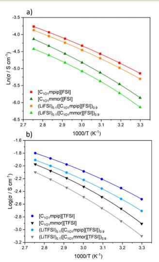
Fig. 5 Temperature dependent ionic conductivity plots of (a) FSI-based ionic liquids and their 10 mol% LiFSI electrolyte solutions and (b) TFSIbased ionic liquids and their 10 mol% LiTFSI electrolyte solutions.
