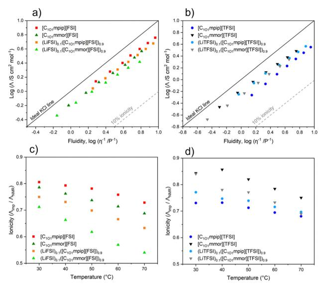
Fig. 7 Walden plot for (a) FSI-based ILs and their electrolyte solutions and (b) TFSI-based ILs and their electrolyte solutions, where  $\Lambda$  is molar conductivity calculated from experimental impedance data and  $\eta^{-1}$  is fluidity, and temperature-dependant ionicity  $I_{HR}$  of (c) FSI-based ILs and their electrolytes and (d) TFSI-based ILs and their electrolytes. Errors were calculated at <4% for all ionicity measurements.
