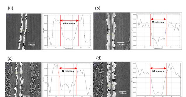
X-ray computed tomography images (1) cross-section of the MEA with mTPN1-TMA membranes at (a) pH-9 (b) pH-10 and (2) cross-section of the MEA with Sustainion membranes at (c) pH-9 (d) pH-10.
