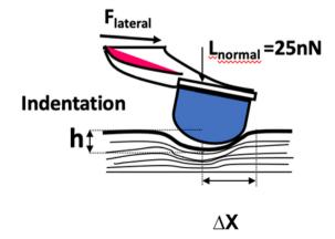
Fig. 3 Tip-surface interaction in SMFM.
