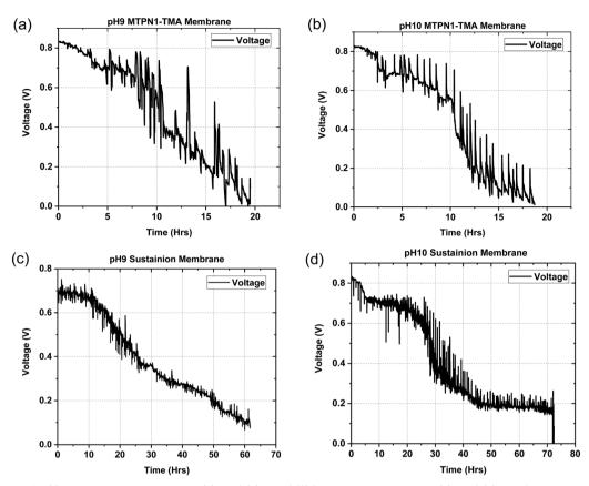
Fig. 9 Durability data for (1) mTPN1-TMA membranes at (a) pH-9 (b) pH-10 (2) Sustainion membranes at (c) pH-9 (d) pH-10 at a constant current density of 0.15 A cm<sup>-2</sup>
