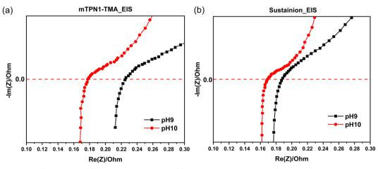
Fig. 10 EIS spectra of AEMFC in inert gas (a) mTPN1-TMA membrane (b) sustainion membrane at pH9 and pH10.
