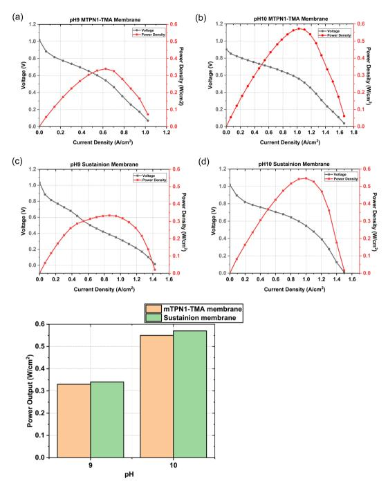
Fig. 8 Polarization Curves for (1) mTPN1-TMA membranes at (a) pH-9 (b) pH-10 and for (2) Sustainion membranes at (c) pH-9 (d) pH-10 (3) Power output vs. pH for mTPN1-TMA membranes and Sustainion membranes
