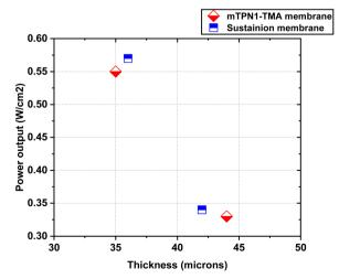
Fig. 12 Power output of both mTP1-TMA membranes and sustainion membranes at different thickness caused by pH.
