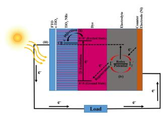
Fig. 9 Typical schematics and working of the dye sensitized solar cells
