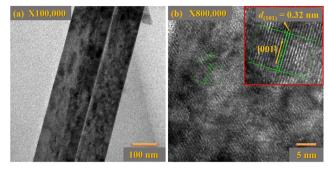
Fig. 4 (a) TEM images of a single TiO<sub>2</sub> NR, and (b) the corresponding HRTEM image of a single TiO<sub>2</sub> NR. The inset image of (b) displays the lattice spacing between (101) planes of rutile phase TiO<sub>2</sub>.
