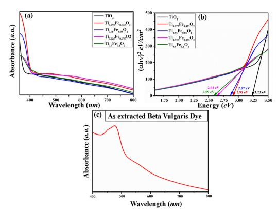
Fig. 6 Absorption spectra of (a)  $Ti_{1-x}Fe_xO_2$  (x = 0 - 0.1) NRs, (b) Tauc plot of the  $Ti_{1-x}Fe_xO_2$  (x = 0 - 0.1) NRs and (c) UV-Visible spectra of the extracted BV dye.
