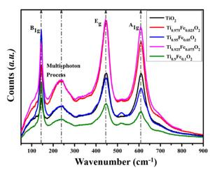
Fig. 8 Raman spectra for tetragonal rutile phase  $Ti_{1-x}Fe_xO_2$  (x = 0-0.1) NRs grown hydrothermally on the FTO substrate.
