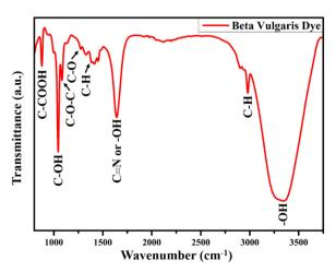
Fig. 7 FT-IR spectrum of the dye extracted from the BV.
