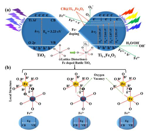
Fig. 1 (a) The process of charge transport involving elevated electrons and VBs of the  $TiO_2$  nanorods with  $Fe^{3+}$  ions of  $Ti_{1-x}Fe_xO_2$  (x = 0-0.1), and (b) schematics of the local topologies of Fe-dopants in the different Fe<sup>4+</sup>, Fe<sup>2+</sup>, and Fe<sup>3+</sup> doped TiO<sub>2</sub> models respectively.  $B^{1-6}$  are the bond lengths of Fe-O bonds and  $\delta$  is the bond angle between Fe-O-Ti and Fe-O-Fe.
