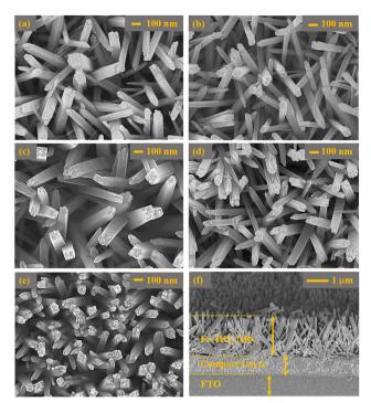
Fig. 3 (a)–(e) FESEM top view image of  $Ti_{1-x}Fe_xO_2$  (x = 0-0.1) NRs grown. (a) Undoped (x = 0) TiO<sub>2</sub> NRs, (b) x = 0.025, (c) x = 0.05, (d) x = 0.075, and (e) x = 0.1 and (f) cross-sectional image of undoped TiO<sub>2</sub> NR arrays.
