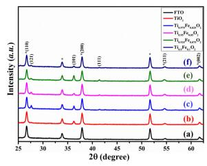
Fig. 2 XRD patterns of the (a) FTO, (b) bare TiO<sub>2</sub>, (c) Ti<sub>0.975</sub>Fe<sub>0.025</sub>O<sub>2</sub>, (d)  $Ti_{0.95}Fe_{0.05}O_2$ , (e)  $Ti_{0.925}Fe_{0.075}O_2$ , and (f)  $Ti_{0.9}Fe_{0.1}O_2$   $TiO_2$  NRs, respectively. \* represents FTO peaks.
