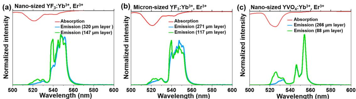
Fig. 3 Normalized UC emission spectra of (a) the nano-sized  $\text{YVO}_4:\text{Yb}^{3+}, \text{Er}^{3+}$ , (b) micron-sized  $\text{YF}_3:\text{Yb}^{3+}, \text{Er}^{3+}$ , and (c) nano-sized  $\text{YF}_3:\text{Yb}^{3+}, \text{Er}^{3+}$ , recorded for different sample thicknesses; ( $\lambda_{\text{ex}} = 975 \text{ nm}$ , bottom) combined with absorption spectra (top) of the obtained products.
