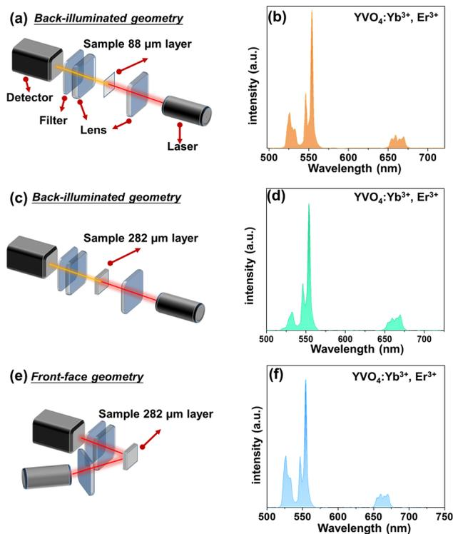
Fig. 2 (a, c and e) Schematic representation of the experimental setup, *i.e.* optical geometry for the UCL measurements and (b, d and f) the corresponding UC emission spectra for the  $\text{YVO}_4:\text{Yb}^{3+}$ ,  $\text{Er}^{3+}$  sample. (a–d) back-illuminated excitation geometry for the  $88 \mu\text{m}$  thick sample (a and b), and for the  $282 \mu\text{m}$  thick sample (c and d); (e and f) front-face excitation geometry for the  $282 \mu\text{m}$  thick sample.
