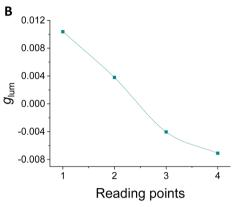
Fig. 10 (A) Method used for reading barcodes at 4 points, from (S,S,P)-1 to (R,R,M)-1. (B) Reading of a barcode with two bands of 32 layers of (S,S,P)-1 to (R,R,M)-1. Average signal of a small wavelength range. See Fig. S28 (ESI+) for raw data
