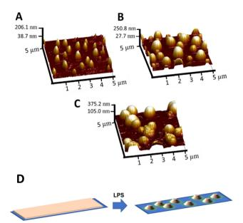
Fig. 4 AFM images, topography in 3D (5  $\mu$ m  $\times$  5  $\mu$ m), of Langmuir films of compound (S,S,P)-1 transferred onto glass slides after subsequent deposition of 8 layers (A), 16 layers (B) and 32 layers (C). Proposed mechanism of liquid phase separation causing the morphology of the films (D).
