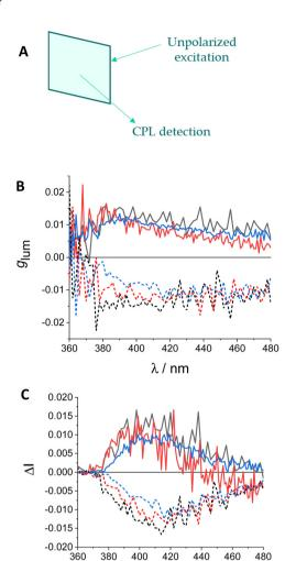
Fig. 8 (A) Method used for measuring CPL values of compounds transferred onto glass slides. (B)  $g_{lum}$  and C)  $\Delta I$  values of (S,S,P)-1 (continuous lines) and (R,R,M)-1 (discontinuous lines) in quartz plates with 8 (black line). 16 (red line) and 32 (blue line) layers. Excitation wavelength: 250 nm.
