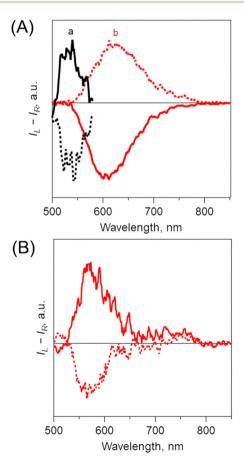
Fig. 6 (A) Circularly polarized luminescence (CPL) spectra of (a) 0Ph-B-BODIPY (monomer) in THF and (b)  $(0Ph-B-BODIPY)_m$  in  $H_2O/THF = 99/1$ (v/v),  $\lambda_{ex}$ : 350 nm. (B) R-(1Ph-B-BODIPY)<sub>m</sub> in H<sub>2</sub>O/THF = 99/1 (v/v),  $\lambda_{ex}$ : 350 nm. Solid and dotted lines correspond to S and R forms, respectively.
