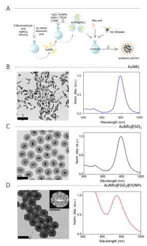
Fig. 1 (A) Schematic representation of the synthesis of AuNR@SiO $_2$ @ IONPs. (B–D) TEM images and normalized (at LSPR maximum) UV-visible spectra for AuNRs (B), AuNR@SiO $_2$  (C), and AuNR@SiO $_2$ @IONPs (D). The inset in (D) shows a single particle imaged using high-angle annular dark field (HAADF) STEM. Scale bars correspond to 200 nm (100 nm in the inset).
