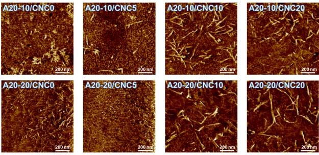
Fig. 3 Tapping-mode AFM phase images of the A20-10/CNC and A20-20/CNC nanocomposites (image size:  $1 \times 1 \mu m$ , scan rate: 1 Hz). These images show the rod-like structures of A20-10 and A20-20 disappear upon CNC loading in PPUs, indicating that a change of hydrogen bonding arrangements from PBLA-PBLA to PBLA-CNC results in phase separation behavior.
