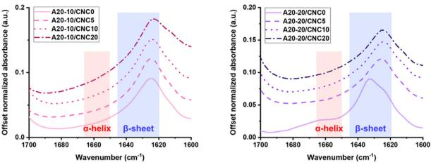
Fig. 2 ATR-FTIR spectra of PPU/CNC nanocomposites as a function of the CNC weight fraction. Peptide secondary structure was identified based on the second derivative in the amide I stretching region (1700-1600 cm<sup>-1</sup>). CNC incorporation into PPUs leads to variations in secondary conformation, disrupting \alpha-helical ordering but promoting intermolecular hydrogen bonding. This finding provides evidence of preferential interactions between the PBLA blocks and CNCs.
