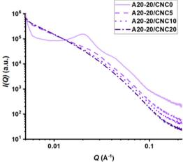
Fig. 4 1D-SAXS profiles of the PPU/CNC nanocomposites with varying PBLA and CNC content collected at room temperature for 30 minutes. The neat PPU matrices (i.e., A20-10/CNC0 and A20-20/CNC0) exhibit a defined scattering peak, whereas the addition of CNC to the matrices results in a reduction or loss of the distinct peak. These results indicate that the introduction of CNCs into PPU matrices modulates long-range ordering and structural hierarchy
