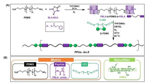
Fig. 1 (A) Synthetic scheme of PPUs (matrix) and (B) building blocks (i.e., matrix and nanofiller) used to design PPU/CNC nanocomposites.
