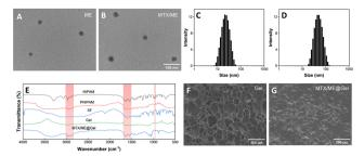
Fig. 1 TEM images of the IL-ME (A) and MTX/ME (15 mg mL $^{-1}$ ) (B) along with their size distributions in (C) and (D). FT-IR spectra of NIPAM, PNIPAM, SF, Gel, and MTX/ME@Gel (E). SEM images of the Gel (F) and MTX/ME@Gel (G).
