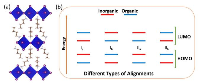
Scheme 1 Schematic diagram of (a) a typical 2D hybrid perovskite structure and (b) different types of intramolecular band alignments in a 2D perovskite.
