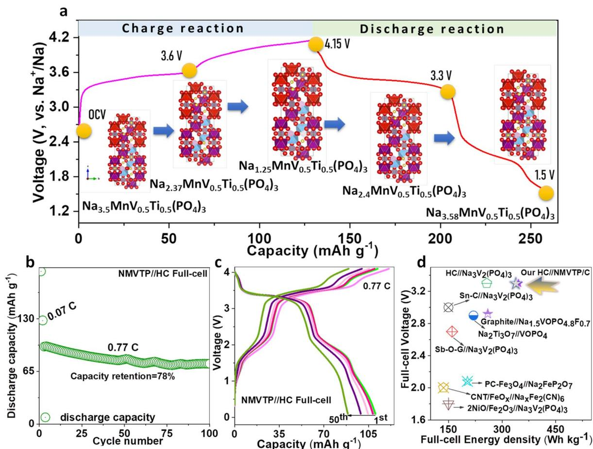
Fig. 6 (a) Schematic illustration of the electrochemical Sodium storage properties of NMVTP cathode. (b) Cyclability profile and (c) selected charge/discharge pattern of the NMVTP/C//HC full-cell at 0.77C (d) voltage and energy density comparison.
