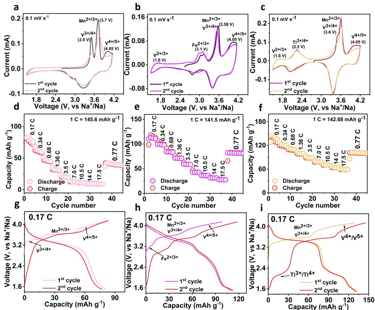
Fig. 2 CV profile at  $0.1 \text{ mV s}^{-1}$  for (a) NMVAP/C, (b) NMVFP/C, and (c) NMVTP/C cathodes. Rate performance acquired at various C rates for (d) NMVAP/C, (e) NMVFP/C, and (f) NMVTP/C cathodes. Charge/discharge pattern at 0.17C for (g) NMVAP/C, (h) NMVFP/C, and (i) NMVTP/C cathodes.
