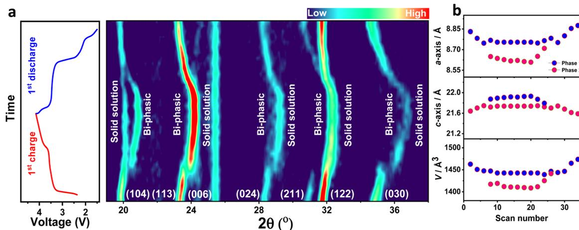
Fig. 5 Sodium storage properties of NMVTP/C cathode (a) the *in situ* 2D contour map profiles along with the equivalent charge/discharge schemes. (b) Lattice parameter and unit cell volume changes upon  $\text{Na}^+$  (de)insertion.
