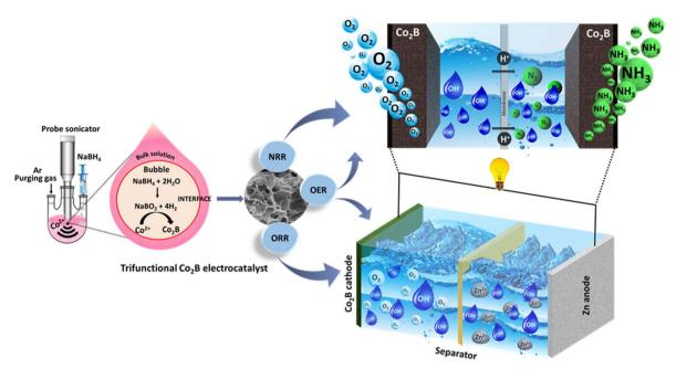
Scheme 1 Schematic representation of the controlled sonochemical synthesis of cobalt boride catalysts signifying trifunctional activity towards NRR/ORR/OER for application in electrochemical ammonia production by as-assembled batteries.
