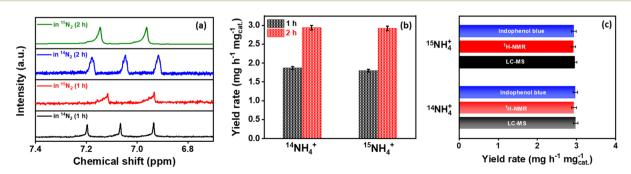
Fig. 2 (a) <sup>1</sup>H-NMR spectrum acquired after NRR isotope labelling experiments using Co<sub>2</sub>B (1:8) catalyst for different time intervals and (b) corresponding yield rates calculated from the same. (c) Bar diagram comparison of <sup>14</sup>NH<sub>4</sub><sup>+</sup> and <sup>15</sup>NH<sub>4</sub><sup>+</sup> yield rates obtained using different quantification methods.
