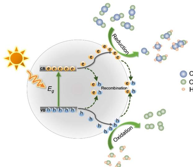
Fig. 2 Schematic illustration of photocatalytic CO<sub>2</sub> reduction.
