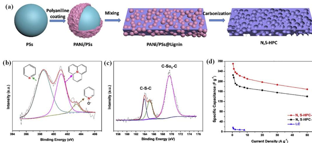
Fig. 9 (a) Schematic preparation procedure for N, S-HPC. High-resolution N1s (b), S2p (c) XPS of N, S-HPC-1. (d) The specific capacitances of the samples at various current densities. Adapted with permission from ref. 164. Copyright 2019 Elsevier.
