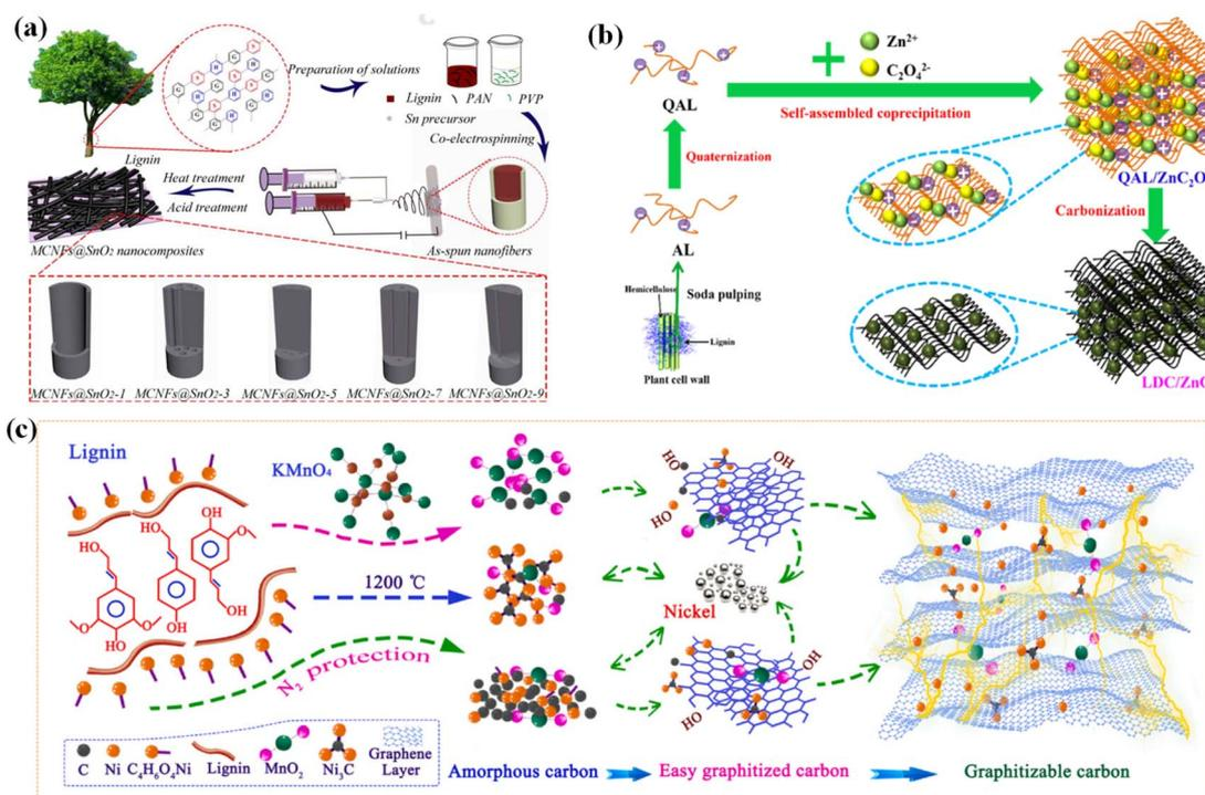
Fig. 7 (a) Schematic procedure for the preparation of MCNFs@ $\text{SnO}_2$  nanocomposites. Adapted with permission from ref. 144. Copyright 2020 Elsevier. (b) Illustration of the fabrication mechanism of the LDC/ZnO materials. Reprinted with permission from ref. 145. Copyright 2019 American Chemical Society. (c) Proposed catalytic graphitization mechanism of Ni. Reprinted with permission from ref. 146. Copyright 2021 Elsevier.
